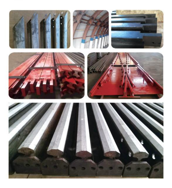
To satisfy the different kinds requirements of our clients, our company procure many kinds of machining equipment, which can carry out secondary machining of the steel rail, such as cutting, drilling, painting, hole-making.etc.
